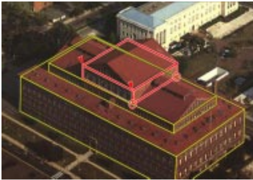
Circles tell you that the object is glued to the one below.
